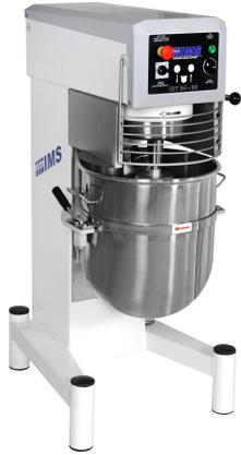
**IBT 42-33** 40 l planetary mixer, stainless steel safety cover, with 3 speed motor (65 –130 –195 rpm). Oil-less planetary system. Equipped with spiral hook, paddle, whisk.
