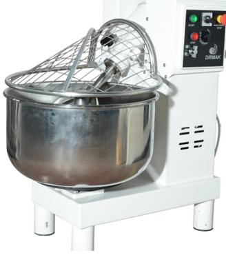
**PET 70** 70 l fork type dough kneader, specially design fork arm, silent operation for all kinds of dough. Long life kneading system is made by endless screw and gear inside a powerful reducer. Bowl, cover and fork arm made of AISI 304 stainless steel.
